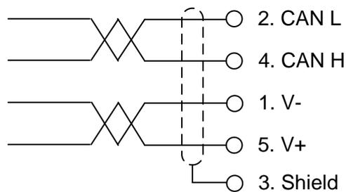
For reliable fieldbus function, line termination must be arranged in both ends of the transmission line. For a G5 Instrument placed at the end of the line, terminate line by placing a 121-ohm resistor between CAN L (pin 2) and CAN H (pin 4).
