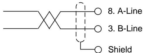
For reliable fieldbus function, line termination must be arranged in both ends of the transmission line. For a G5 instrument, at the end of the cable, a connector with line termination should be used. For all other G5 Instruments, connection without line termination should be used.
